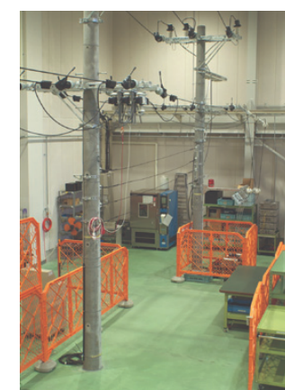
Simulated power pole for electricity distribution line
